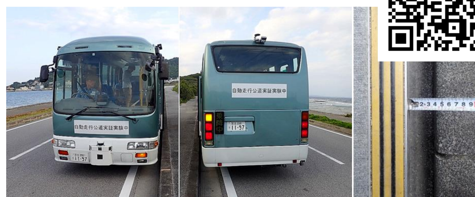
(a) Precision docking control (b) Accuracy of precision docking Experimental results of precision docking
